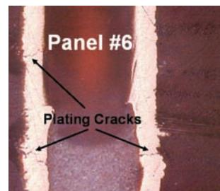
Figure 15. Sample of Barrel Crack Failure, Advanced FR4B.
