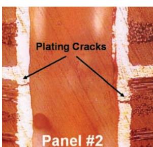
Figure 13. Sample of Barrel Crack Failure, Standard FR4.
