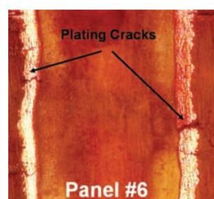
Figure 14. Sample of Barrel Crack Failure, Advanced FR4A.
