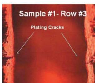
Figure 9. Sample of Barrel Crack Failure.
