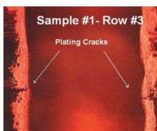
Figure 8. Sample of Barrel Crack Failure.
